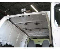
Be sure to tape harnesses to roof in approximate locations that accessories are being installed in Kwik kit. This will vary between the different model kits.
